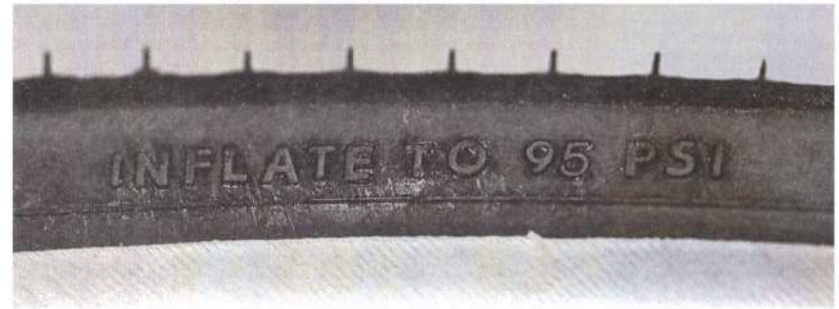
Tires should be kept inflated to the maximum pressure recommended by the manufacturer. This pressure is stamped on the side of the tire.
