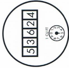
Direct water meter
