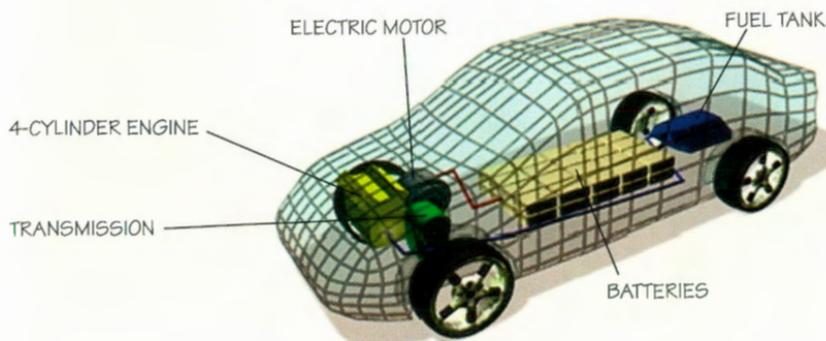
**Gasoline-electric parallel hybrid drive train**
