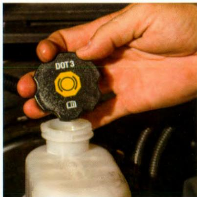
Checking the brake fluid
