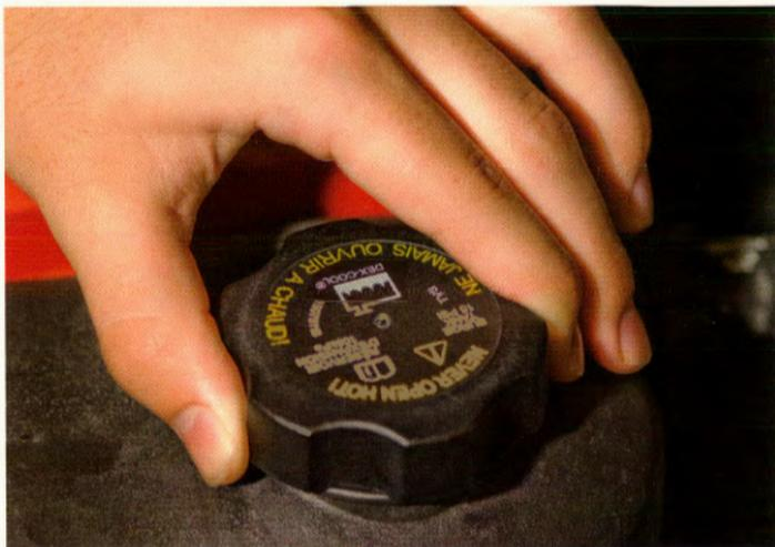
**Remove the radiator cap only if the engine is cool.**
