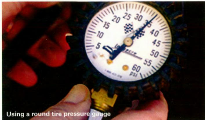
Using a round tire pressure gauge
