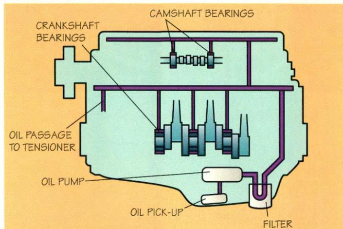
**Lubrication system components**
