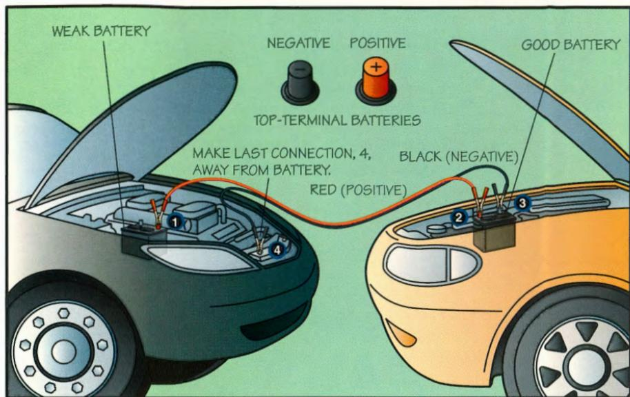
Correct jumper cable connections
