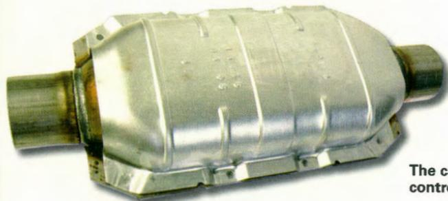
The catalytic converter controls exhaust emissions.
