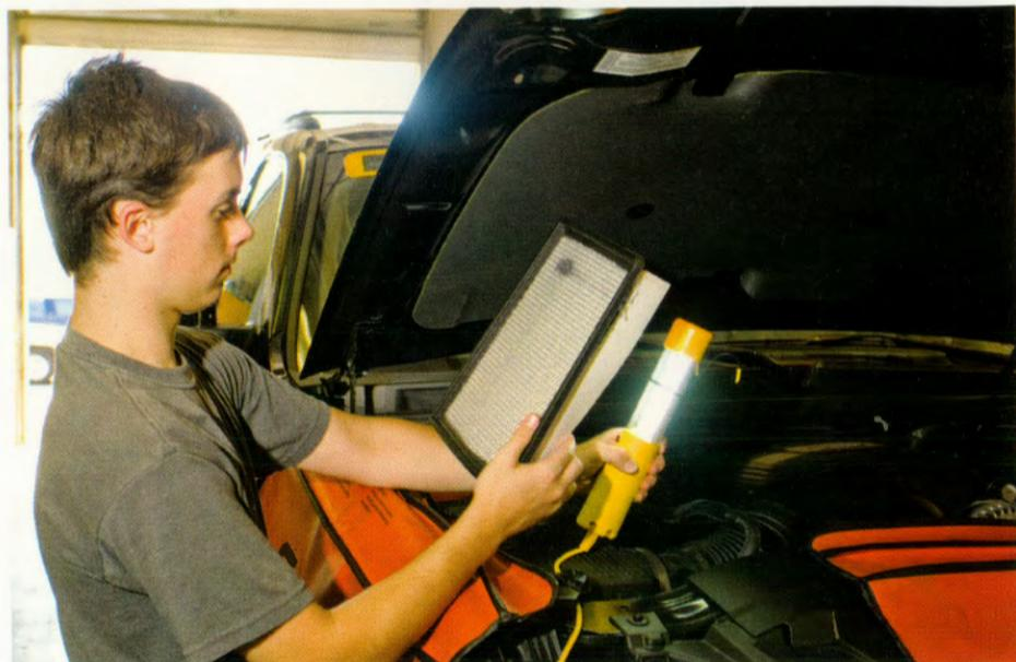
Checking the air filter
