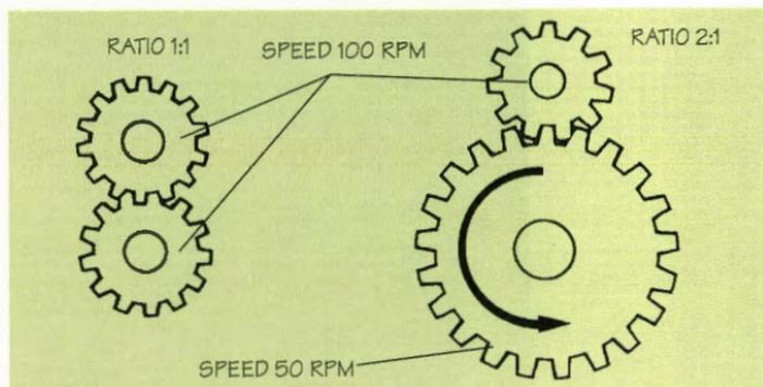
**The ratio between the size of two gears affects the torque the gears generate.**
