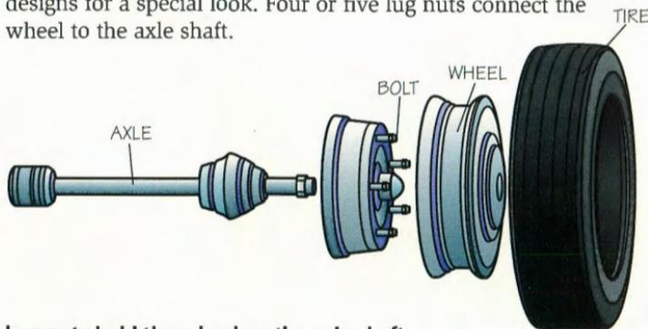
Lug nuts hold the wheel on the axle shaft.
