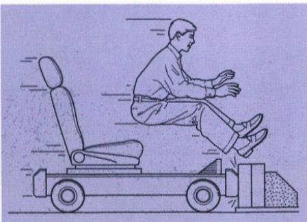
**Why are safety belts necessary? Take this example: A man is riding a simple vehicle at any speed, and the vehicle stops suddenly. The rider does not stop until he hits another object. Had a safety belt been in place, the rider would have stopped while still in the seat.**
