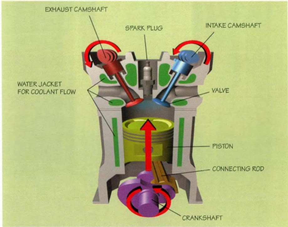
Combustion chamber components
